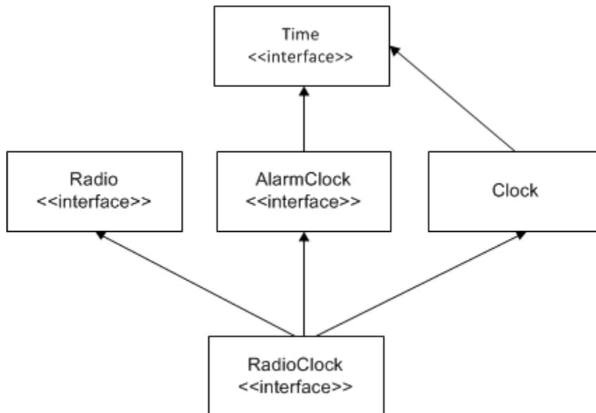
*A Class using implementation and interface inheritance.*
