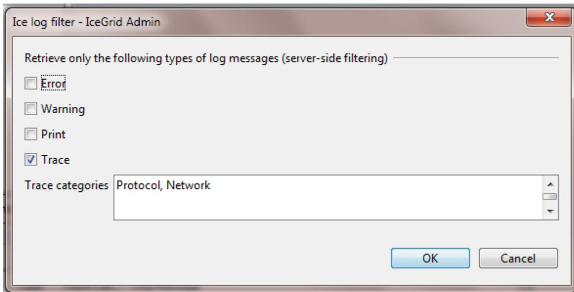
This dialog allows you to filter the log messages sent by the monitored Ice applications. All the filtering is done in this remote Ice application.
