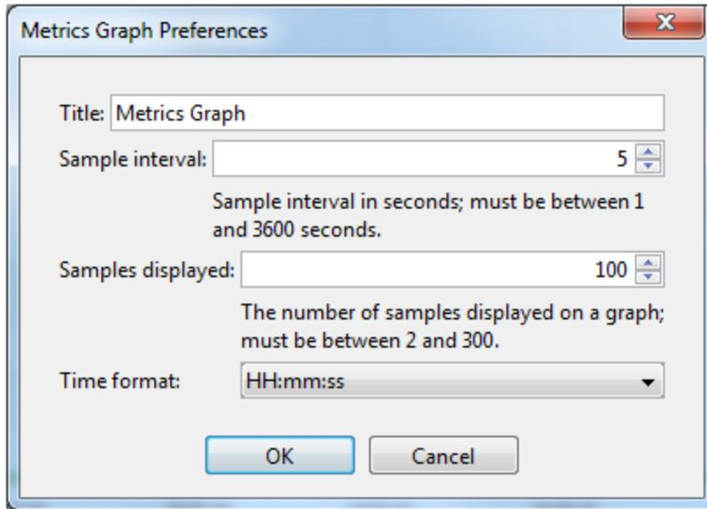
For each metric plotted in a Metrics Graph, IceGrid Admin retrieves the corresponding value every `Sample interval` seconds (by default every 5 seconds), and displays `n` values (`n = 120` by default). `Sample interval` times `Samples displayed` correspond to the time period represented on a graph; by default, it is  $5s * 120 = 10$  minutes.
