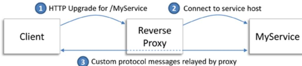
The client connects to the HTTP server and sends an HTTP request to upgrade the existing connection to support WebSocket. The message includes a resource path, such as `/MyService` in the example above, that the HTTP server translates into a target back-end service. The HTTP server establishes its own connection to the service and then relays messages between the client and the service. The service is an Ice server listening on a WS or WSS endpoint.
