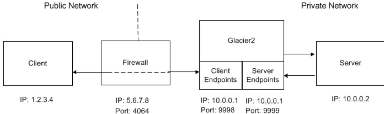
The Glacier2 router in the example above has both of its endpoints in the private network and its host requires only one IP address, unlike the example we showed in the discussion of [bidirectional connections](#) in which the Glacier2 host straddled both networks.
