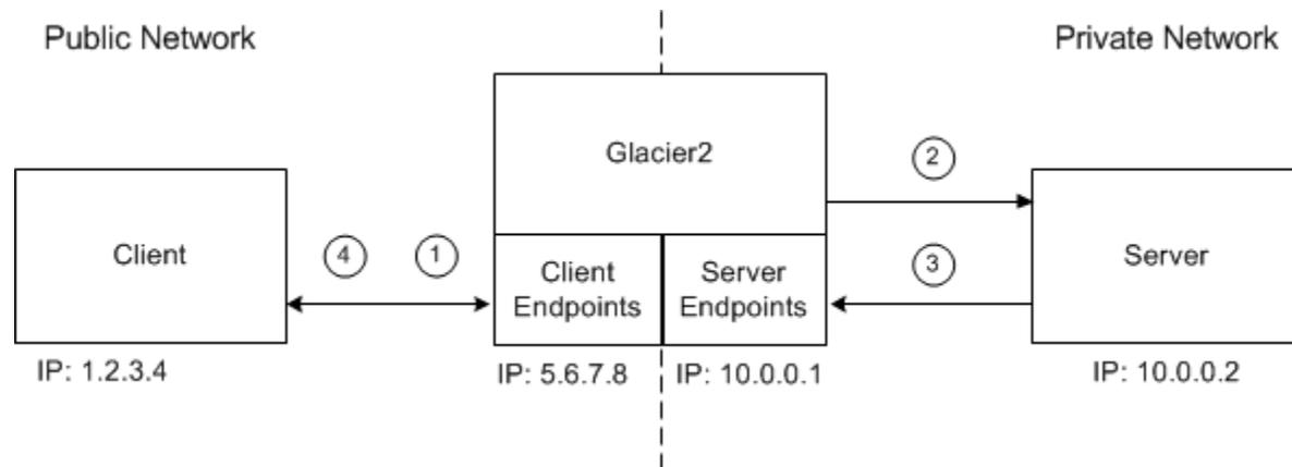
1. The client has a routed proxy for the server and makes an invocation. A connection is established to the router's client endpoint and the request is sent to the router.
