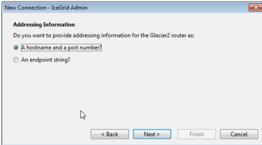
Step 3: Enter the hostname of the Glacier2 router, leave the port number empty to use the default Glacier2 port number (4063 for TCP and 4064 for SSL), and select SSL for the protocol:
