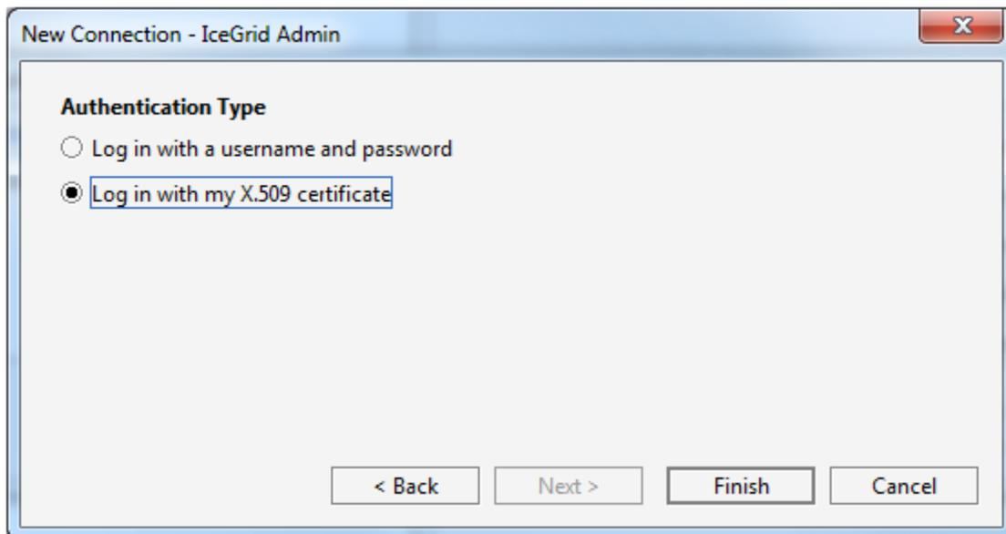
Step 9: Click `Finish` to save the connection and connect to the IceGrid registry. Unless we entered (and therefore saved) the X.509 key password with the connection, we are prompted for this password:
