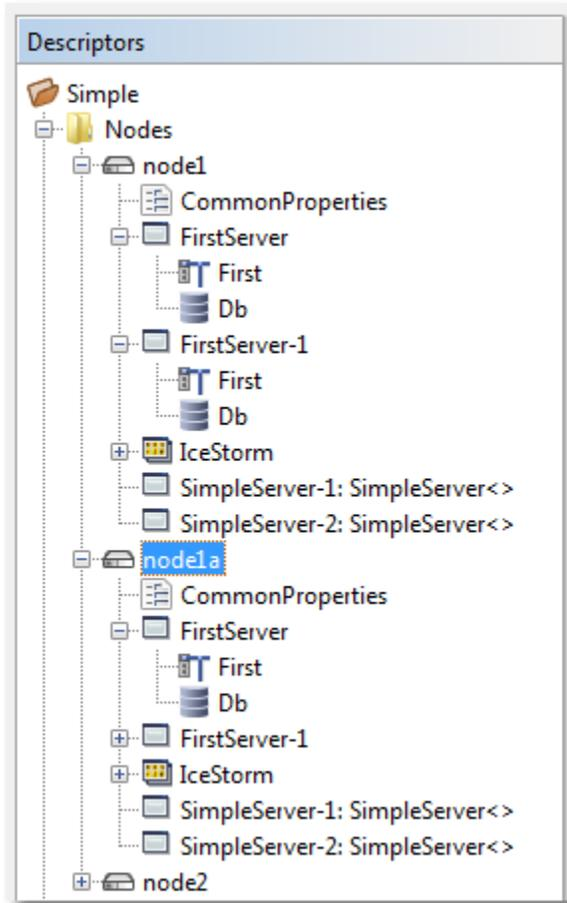
After pasting a sub-tree, you typically need to check and edit the new elements to avoid any duplicate server IDs, adapter IDs etc.
