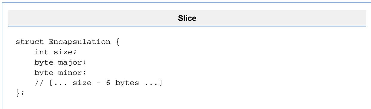
The `size` member specifies the size of the encapsulation in bytes (including the `size`, `major`, and `minor` fields). The `major` and `minor` fields specify the [encoding version](#) of the data contained in the encapsulation. The version information is followed by `size-6` bytes of encoded data.
