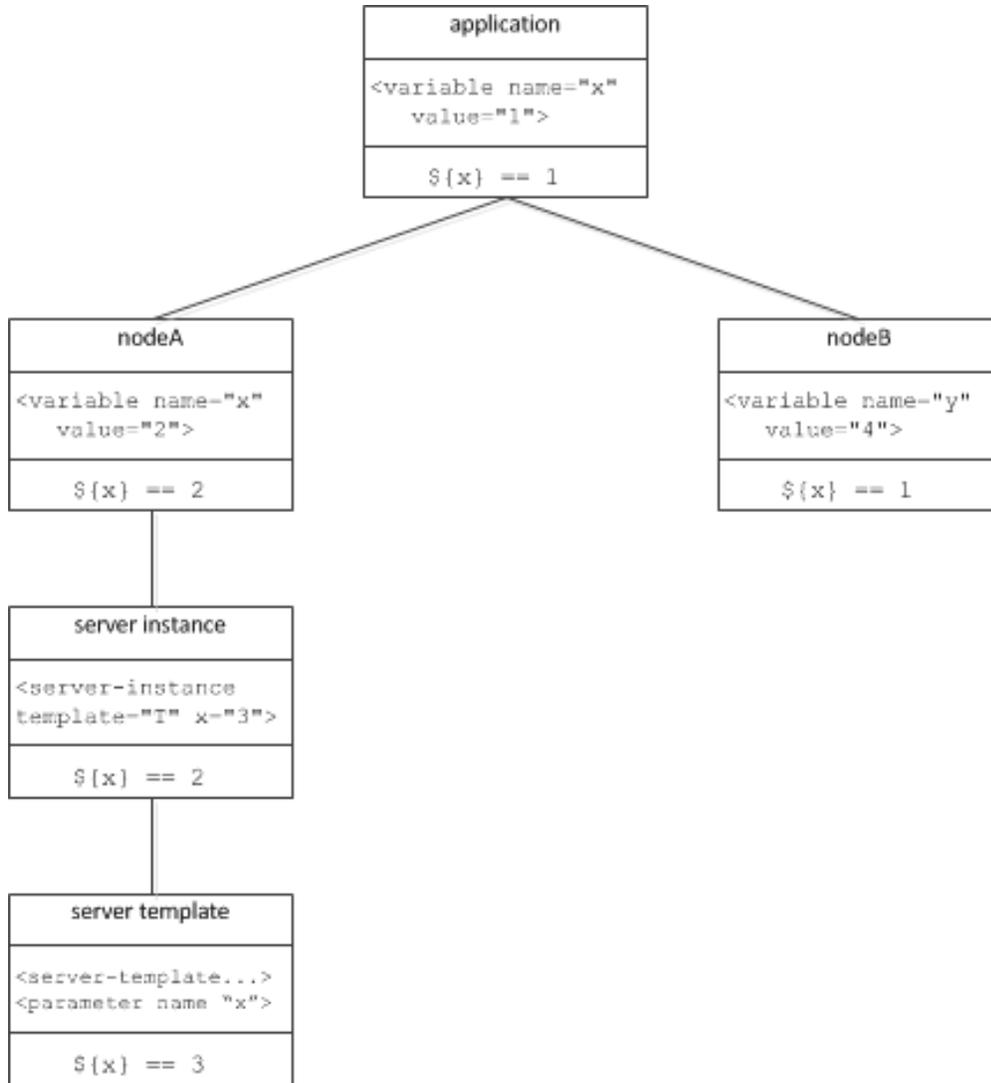
In this diagram, the variable `x` is defined at the application level with the value 1. In node A, `x` is overridden with the value 2, whereas `x` remains unchanged in node B. Within the context of node A, `x` continues to have the value 2 in a server instance definition. However, when `x` is used as the name of a template parameter, the node's definition of `x` is overridden and `x` has the value 3 in the template's scope.
