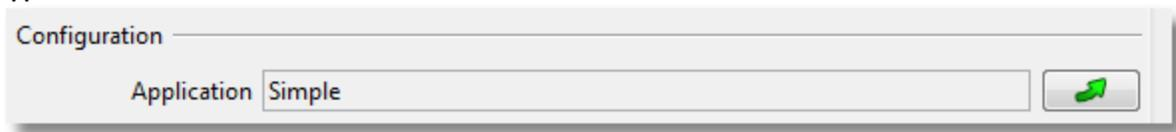
The name of the application containing this server's definition. The button on the right shows the server definition in an Application tab.
